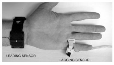
Figure 2. Wrist and Finger PPG Sensors [21]
